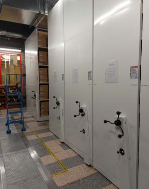
Example of rolling racking system (manually operated) at The Secret Collection, Paisley
